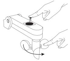
With the **SEL** button position the LED TEST will begin to flash this. Press the **SET** button for more than 1 second and the LED stays ON.
