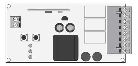
Control board MC8, for automation of awnings, with the possibility of connecting the timer light presence, with operation via remote control and Sensor Wireless (sun/wind/rain).
